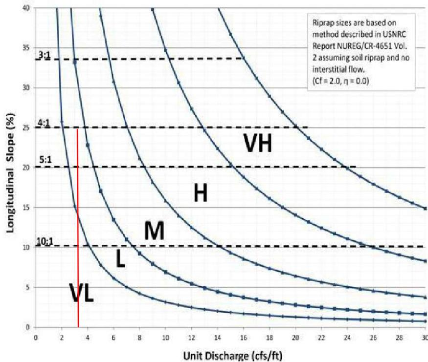
Spillway Q100 = 16.1 cfs (Undetained DP-A1A)
