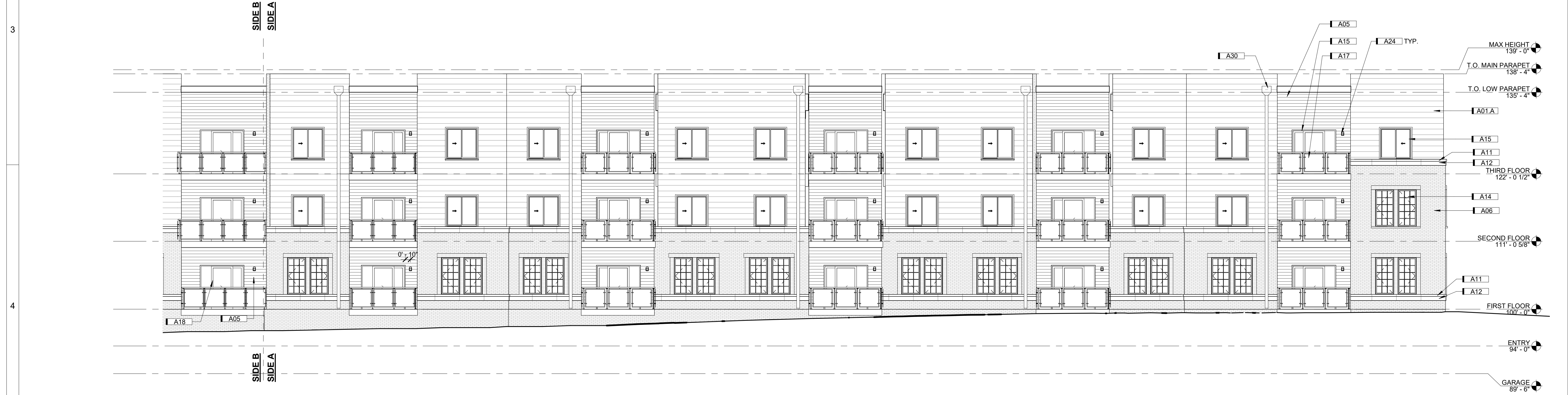
A4 WEST ELEVATION - SIDE B 1/8" = 1'-0" 0 12'
