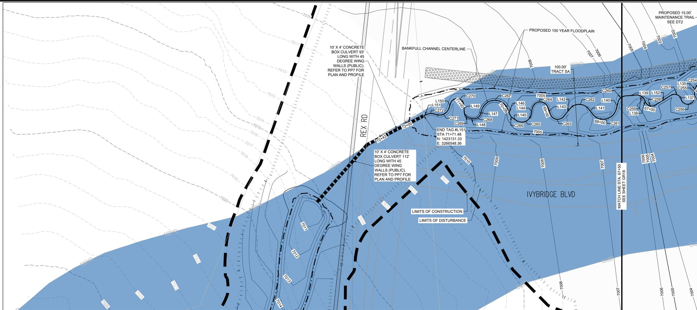
10' X 4' CONCRETE BOX CULVERT 93' LONG WITH 45 DEGREE WING WALLS (PUBLIC). REFER TO PP7 FOR PLAN AND PROFILE
