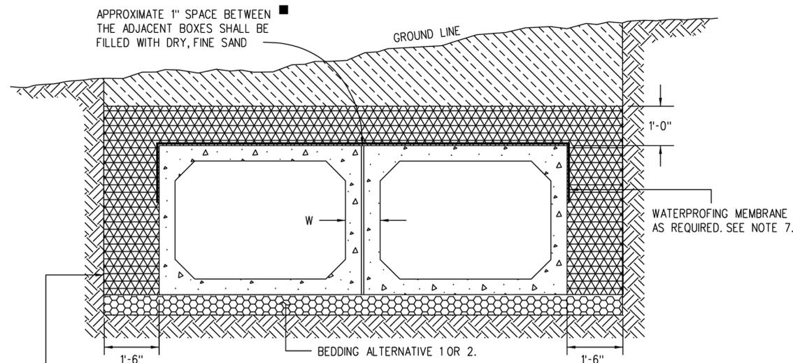
EXCAVATION & BACKFILL WILL BE MEASURED AND PAID FOR TO THIS LINE IN ACCORDANCE WITH SECTION 206.
