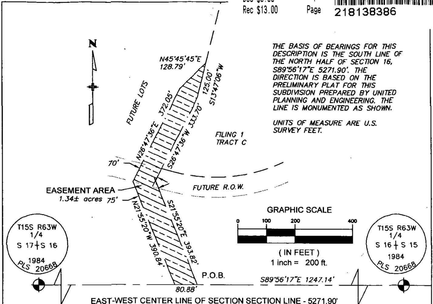
THE BASIS OF BEARINGS FOR THIS DESCRIPTION IS THE SOUTH LINE OF THE NORTH HALF OF SECTION 16, S89°56'17\"/>
