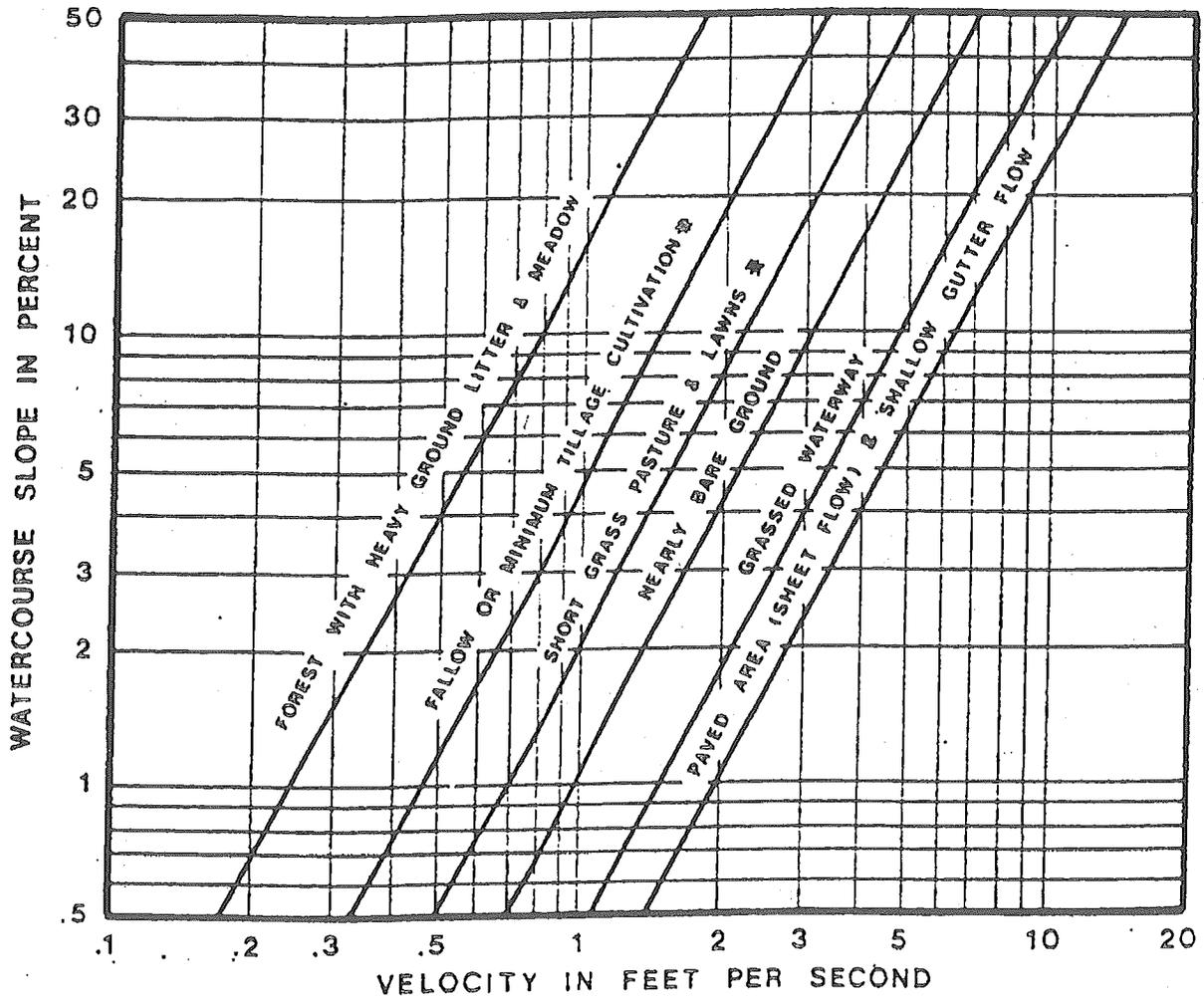
FIGURE 3-2. ESTIMATE OF AVERAGE FLOW VELOCITY FOR USE WITH THE RATIONAL FORMULA.
