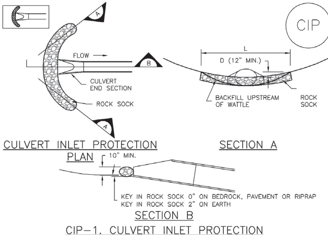
CULVERT INLET PROTECTION INSTALLATION NOTES
