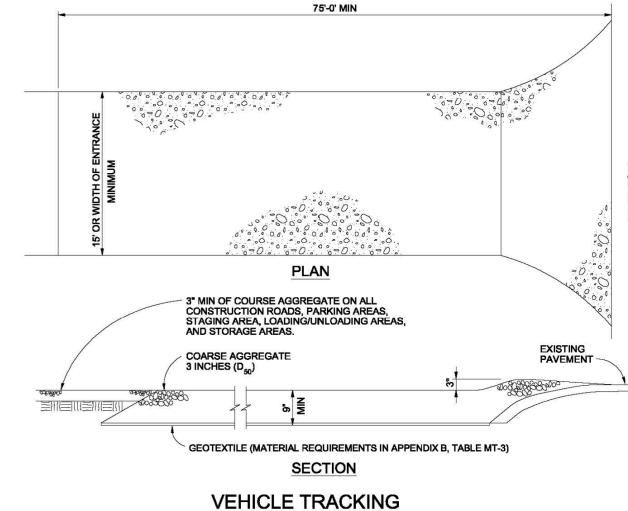
VEHICLE TRACKING NOTES INSTALLATION REQUIREMENTS 1. ALL ENTRANCES TO THE CONSTRUCTION SITE ARE TO BE STABILIZED PRIOR TO CONSTRUCTION
