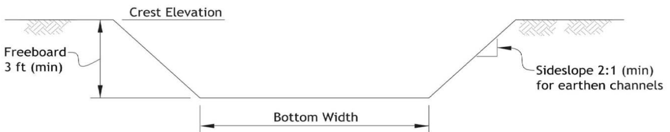
Spillway Section
