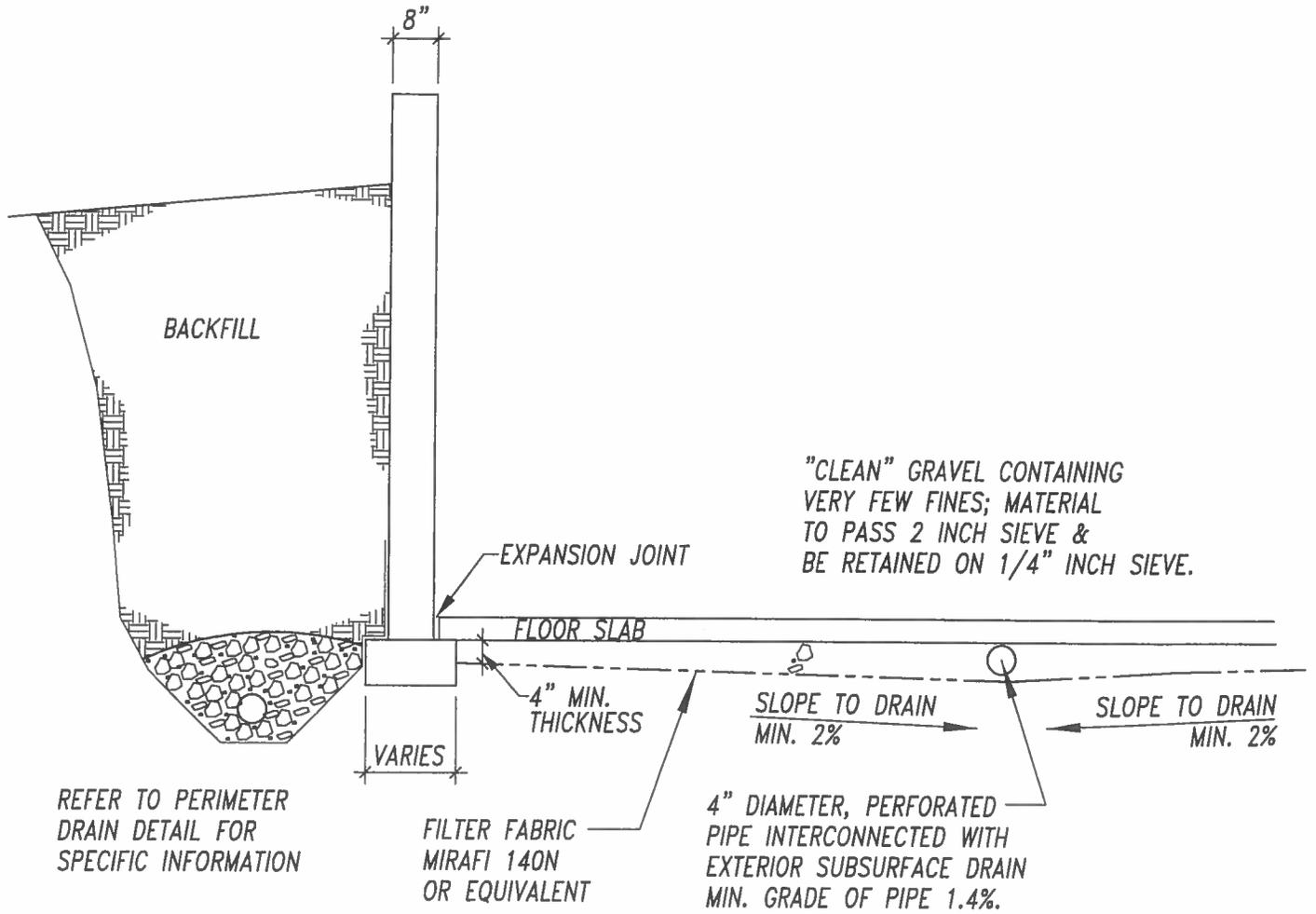
A:\11e\_Detail\RoomDrains\UNDERSLAB CAPILLARY BREAK DRAIN.dwg, Layer:1, 6/12/2007, 12:11:56 PM, 1/48
