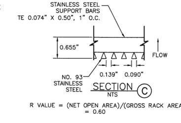
FIGURE OS-5 TYPICAL OUTLET STRUCTURE WITH WELL SCREEN TRASH RACK
