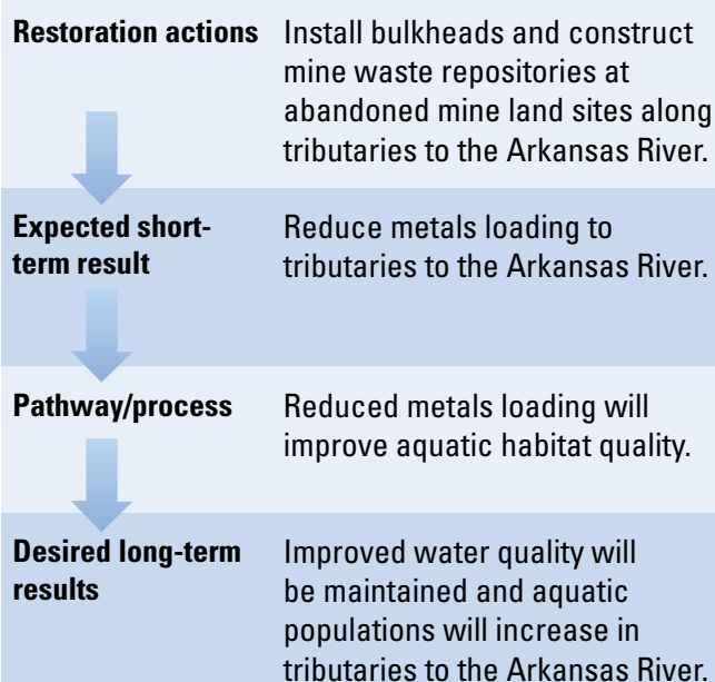
FIGURE 3.16. REMEDIATION OF ACID MINE DRAINAGE IN TRIBUTARIES TO THE ARKANSAS RIVER – LOGIC MODEL
