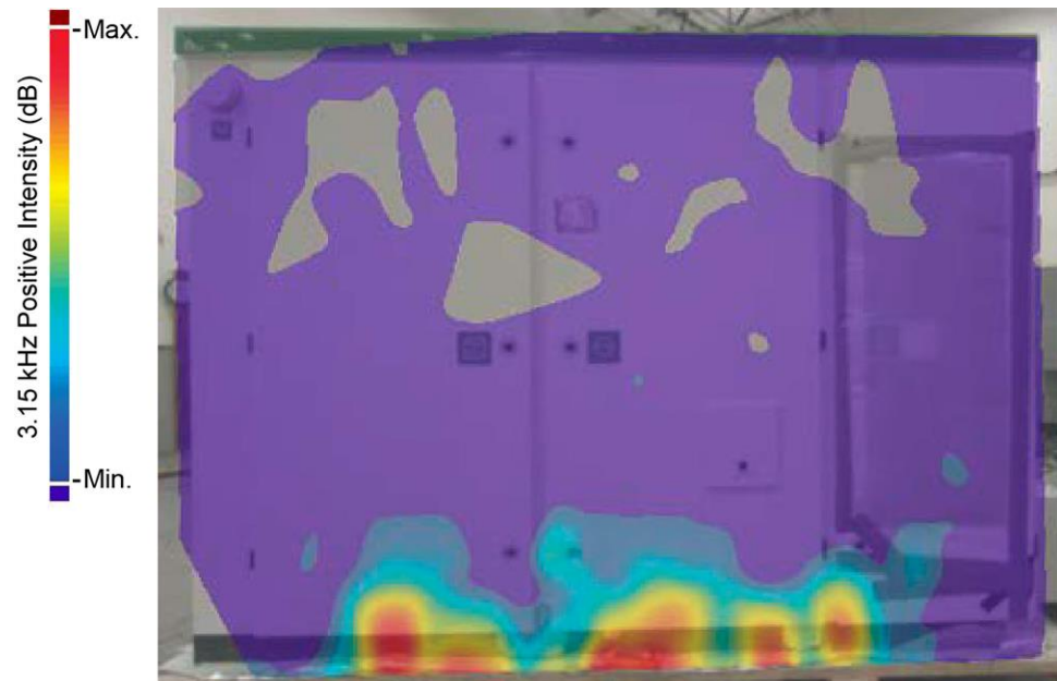
Figure 4 LV and Communications end (3.15 kHz, switching frequency)
