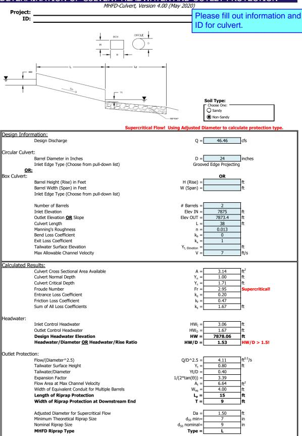
Please revise design to meet criteria regarding supercritical flow and froude number less than 1. Or provide inlet protection calculations/design for the culvert.
