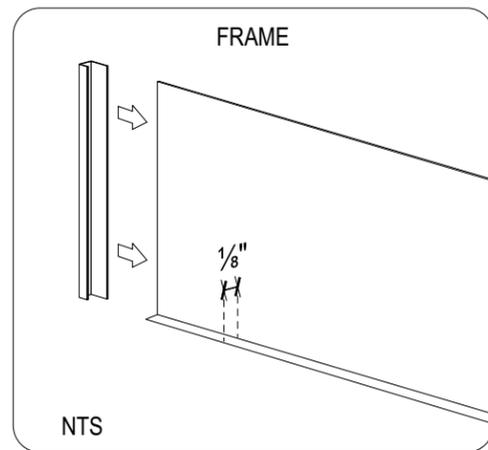
..040" PRECOAT ALUMINUM WITH VHB TAPE ONTO EXISTING WINDOW MULLION
