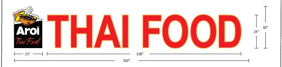
Aluminum Custom Channel White Plex Face Print and Vinyl Overlay Black Trim Cap LED Illumination Raceway Mounted Aluminum Channels Red Plex Faces Gold Trim Cap LED Illumination Raceway Mounted
