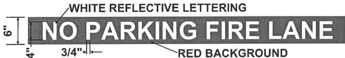
5. Fire lane signs as specified shall be posted on both side of fire apparatus access roads that are 20 to 26 feet wide.
