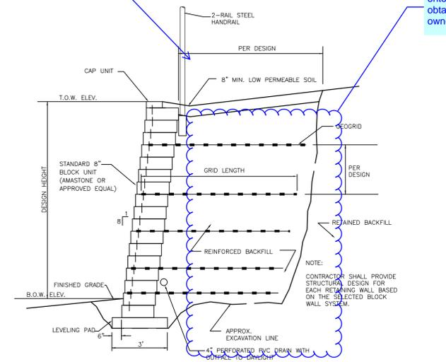
**MODULAR BLOCK RETAINING WALL DETAIL (F)**
