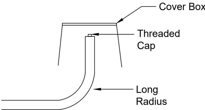
FLUSHING PORT DETAIL
