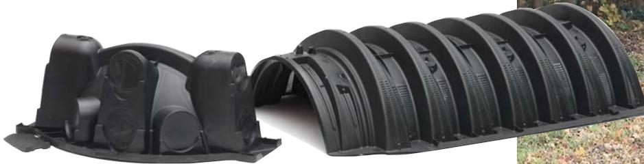
The Quick4® Standard Chamber fits in a 36" wide trench and is ideal for curved or straight systems. It features the patent-pending Contour Swivel Connection™ which permits turns up to 15°, right or left. The MultiPort™ endcap allows multiple piping options and eliminates pipe fittings. The chamber's four-foot length provides optimal installation flexibility.
