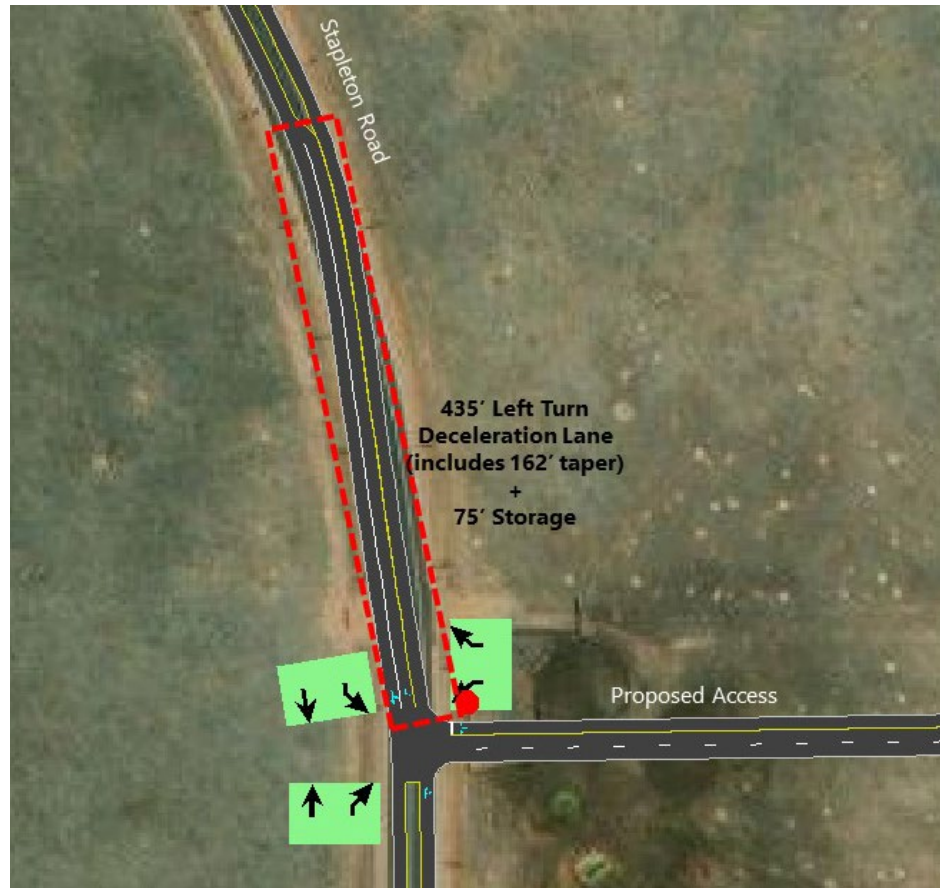
FIGURE 7: RECOMMENDED LEFT TURN LANE
