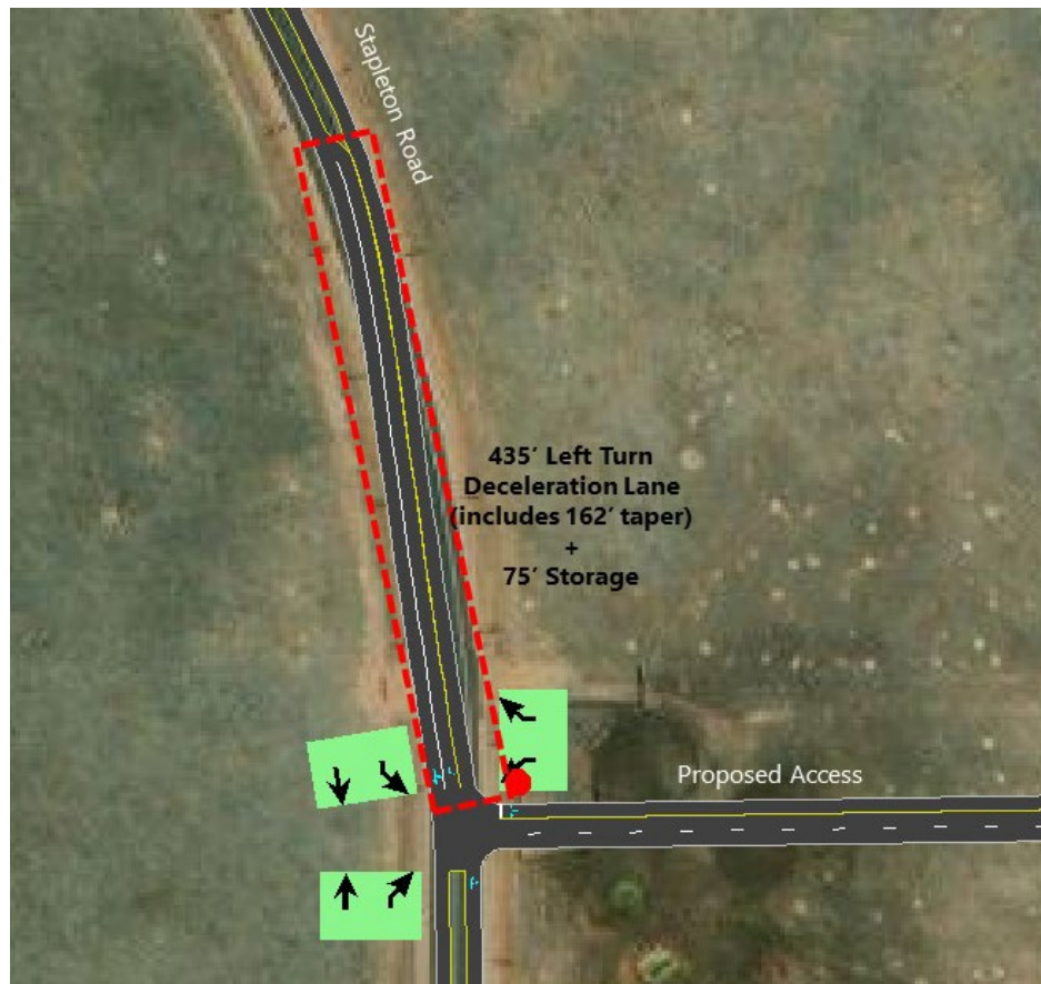
FIGURE 8: RECOMMENDED LEFT TURN LANE
