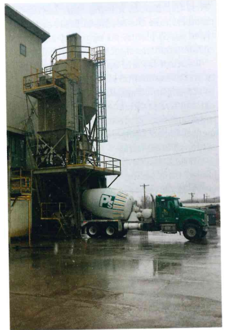
Drivers keep trucks clean, knowing their drums are rolling Pete Lien & Sons billboards. Drums bear alternating colored tick marks so drivers can easily verify rotation direction and avoid accidental discharge.
