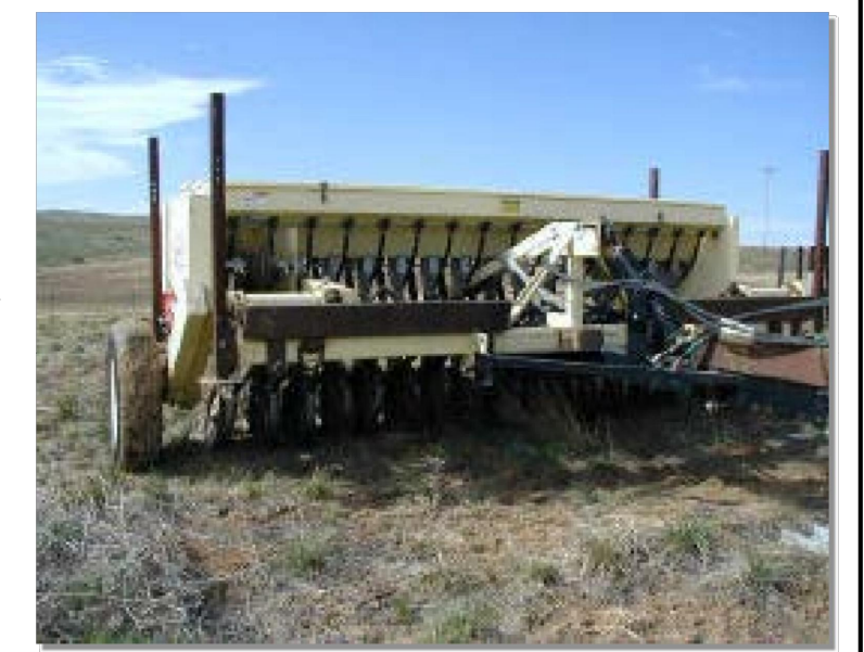
Photograph TS/PS-1. Equipment used to drill seed. Photo courtesy of Douglas County.
