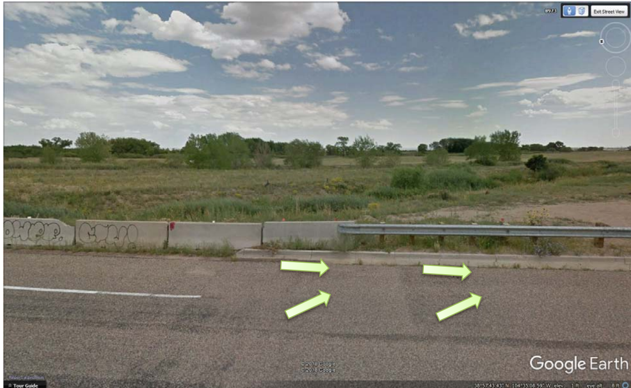
Google Streetview at the upstream end of the gutter line (south side of Bennet Ranch drainageway crossing). Transition from block to 6 inch curb.
