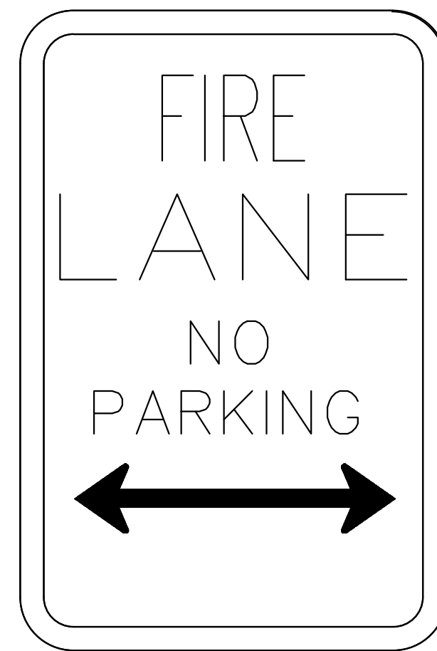
FIRE LANE SIGNAGE DETAIL NOT TO SCALE
