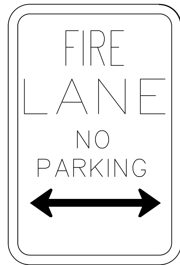
FIRE LANE SIGNAGE DETAIL NOT TO SCALE
