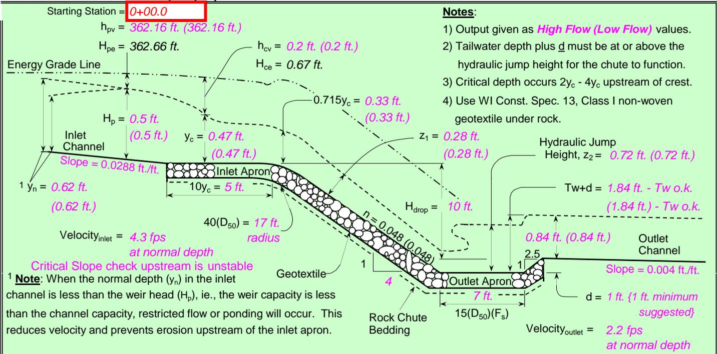
**1 Note:** When the normal depth ( $y_n$ ) in the inlet channel is less than the weir head ( $H_p$ ), i.e., the weir capacity is less than the channel capacity, restricted flow or ponding will occur. This reduces velocity and prevents erosion upstream of the inlet apron.
