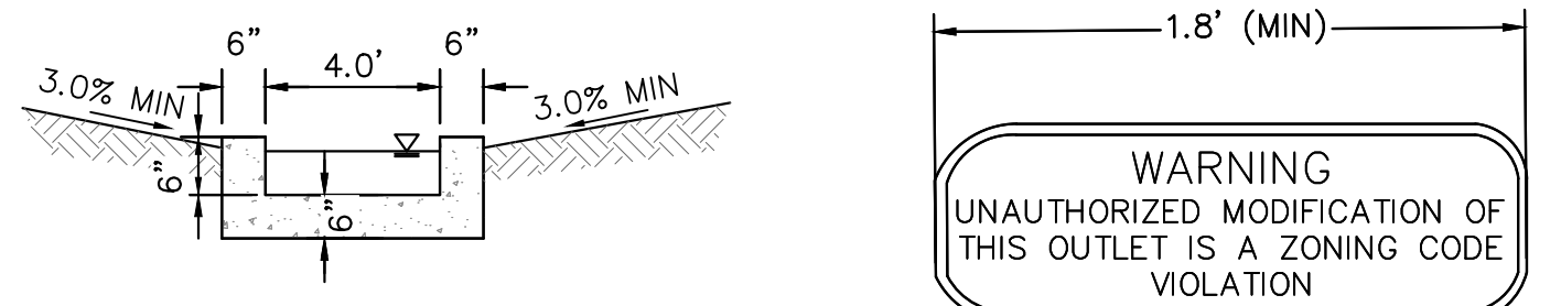
CONCRETE TRICKLE CHANNEL 1"=5' * CONTRACTOR TO INSTALL CONTROL JOINTS @ 10' SPACING OUTLET SIGNAGE N.T.S. OUTLET SIGNAGE NOTES 1. SIGN SHALL BE A MINIMUM OF 0.75 SQUARE FEET AND SHALL BE ATTACHED TO THE OUTLET OR POSTED NEARBY.
