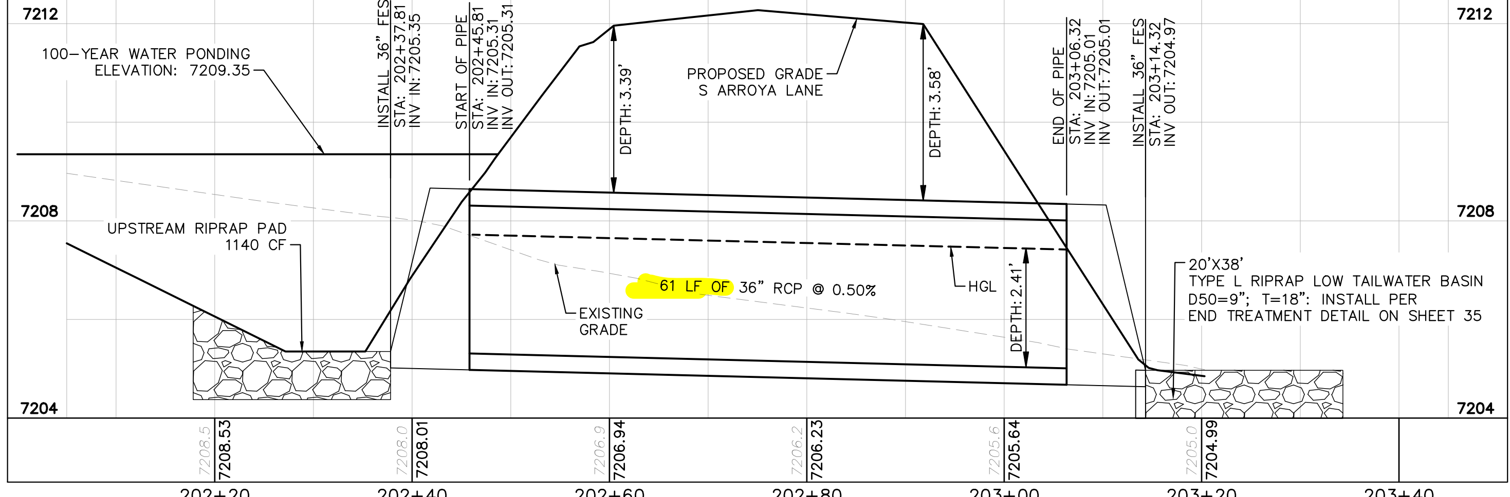
CULVERT 2 (3) - DP10 PROFILE VIEW
