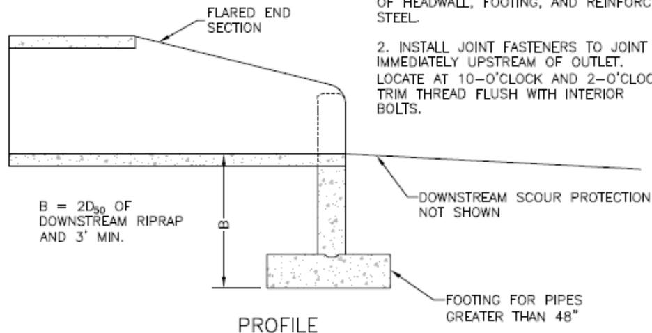
2. INSTALL JOINT FASTENERS TO JOINT IMMEDIATELY UPSTREAM OF OUTLET. LOCATE AT 10-O'CLOCK AND 2-O'CLOCK. TRIM THREAD FLUSH WITH INTERIOR BOLTS.
