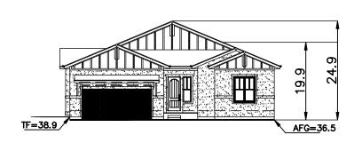
284.1 C ELEVATION 1 STORY AVERAGE FINISH GRADE = (AFG) AFG = <u>38.1+37.8(2)+37.2+36.9+35.1+32.6</u> = 36.5 BUILDING HEIGHT = 17.5 + (TF - AFG) =
