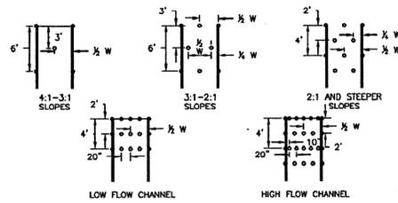
STAKING PATTERNS BY SLOPE OR CHANNEL TYPE
