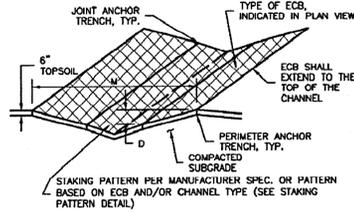
ECB-2. SMALL DITCH OR DRAINAGE WAY
