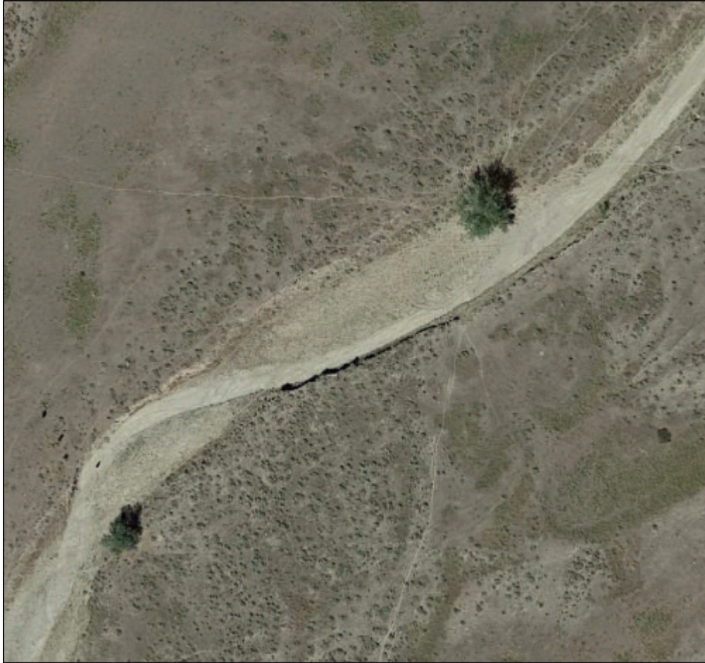
Figure 4-3. Representative Image of Sand-Silt Channel, n = 0.032
