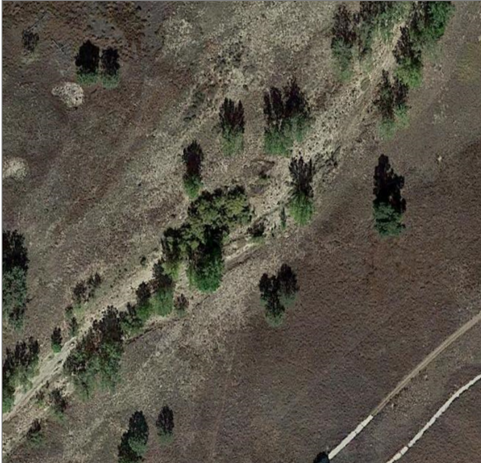
Figure 4-4. Representative Image of Vegetated Streambed, Light to Medium, n=0.040
