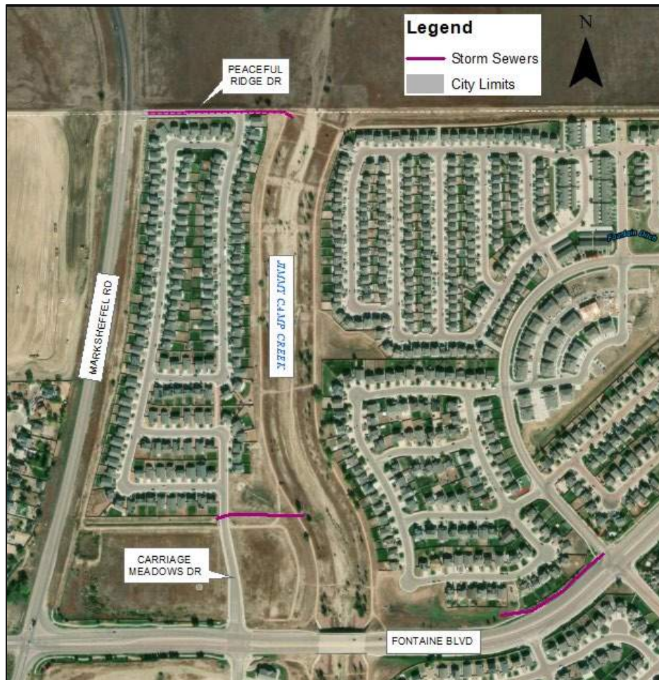
Figure 4-7. Jimmy Camp Creek Storm Sewer Locations
