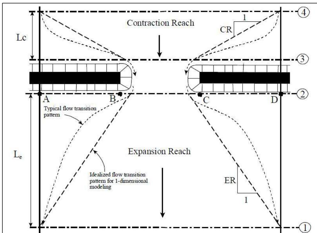
Figure 4-2. Cross Section Locations for Hydraulic Crossings
