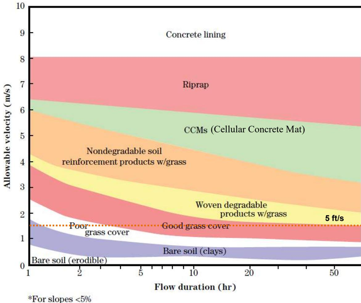
Figure 5-2. Effect of flow duration on allowable velocities for various channel linings from NRCS (2007)
