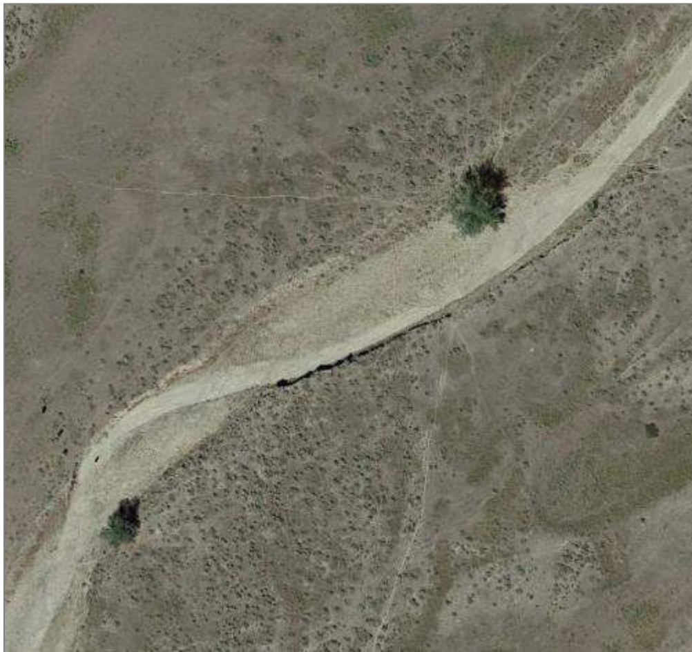
Figure 3-3. Representative Image of Sand-Silt Channel, n = 0.032
