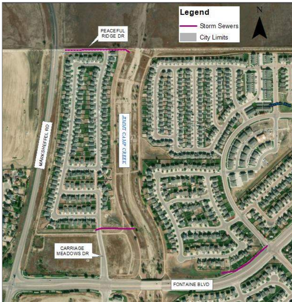
Figure 3-7. Jimmy Camp Creek Storm Sewer Locations
