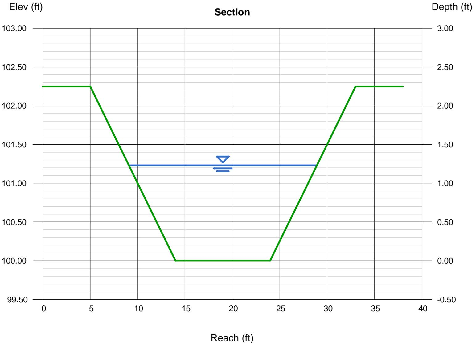
Emergency Spillway Overflow (Triple Type C Grate)
