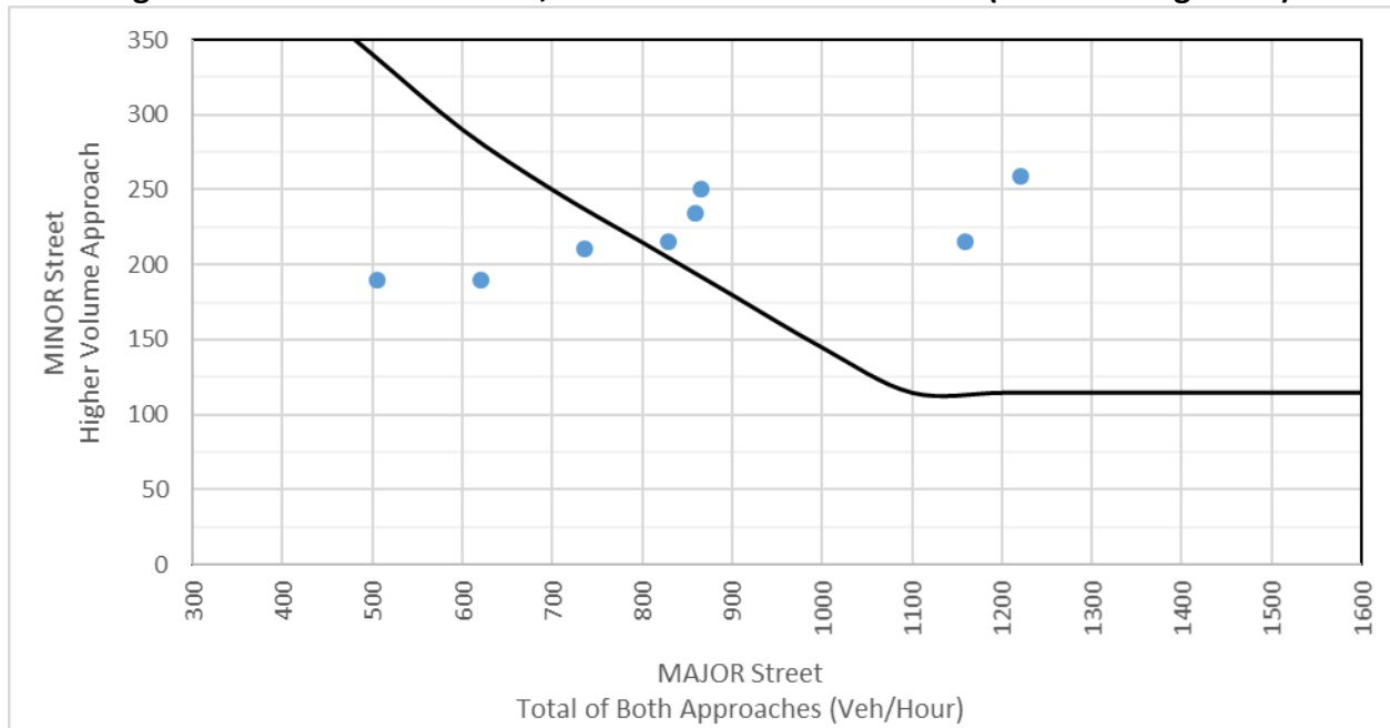
Figure 10: MUTCD Warrant 2, Four-Hour Vehicular Volume (2019 Existing + Site)
