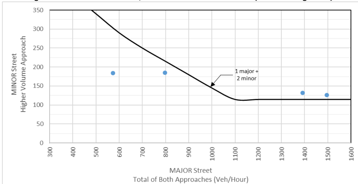
Figure 12: MUTCD Warrant 2, Four-Hour Vehicular Volume (2019 Existing + Site)
