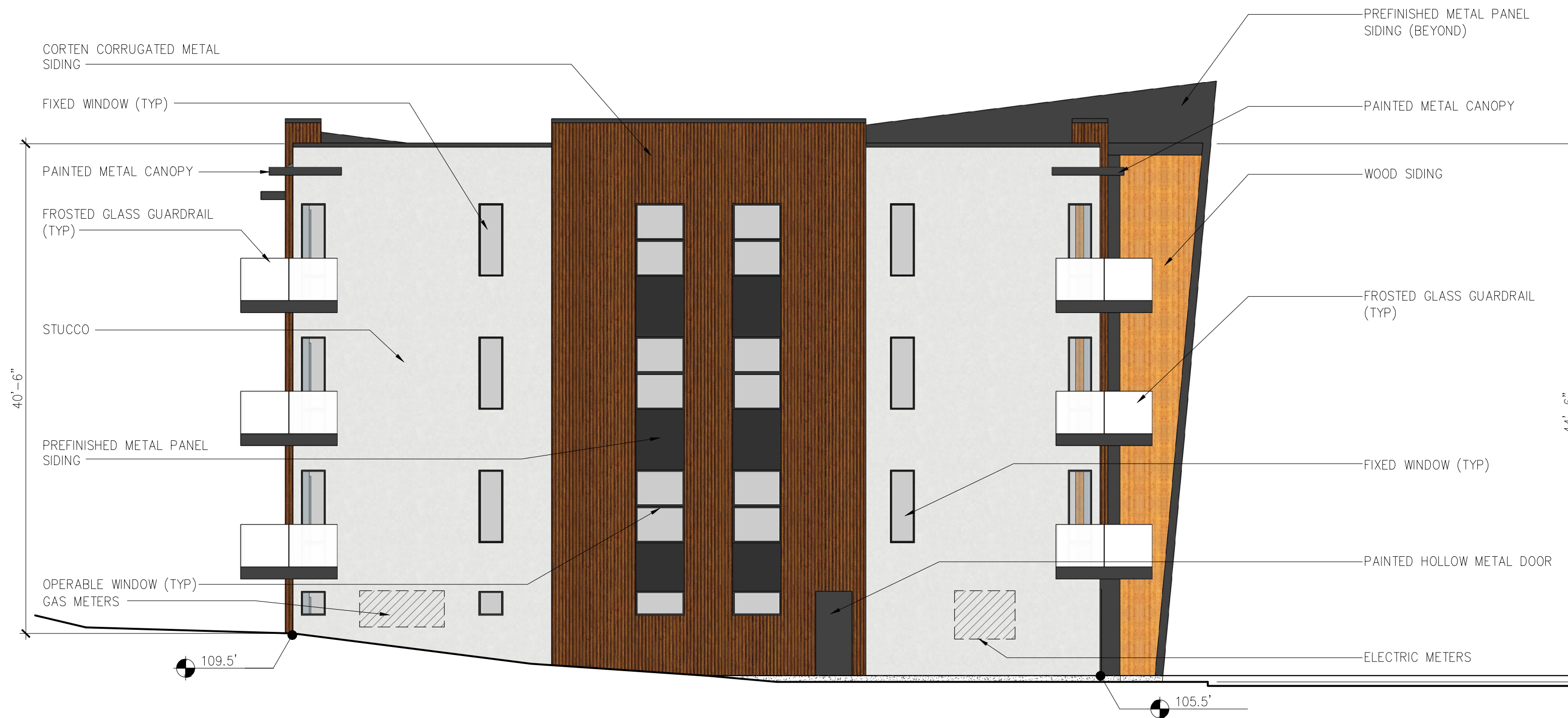
2 SOUTH EXTERIOR ELEVATION 1/8"=1'-0"
