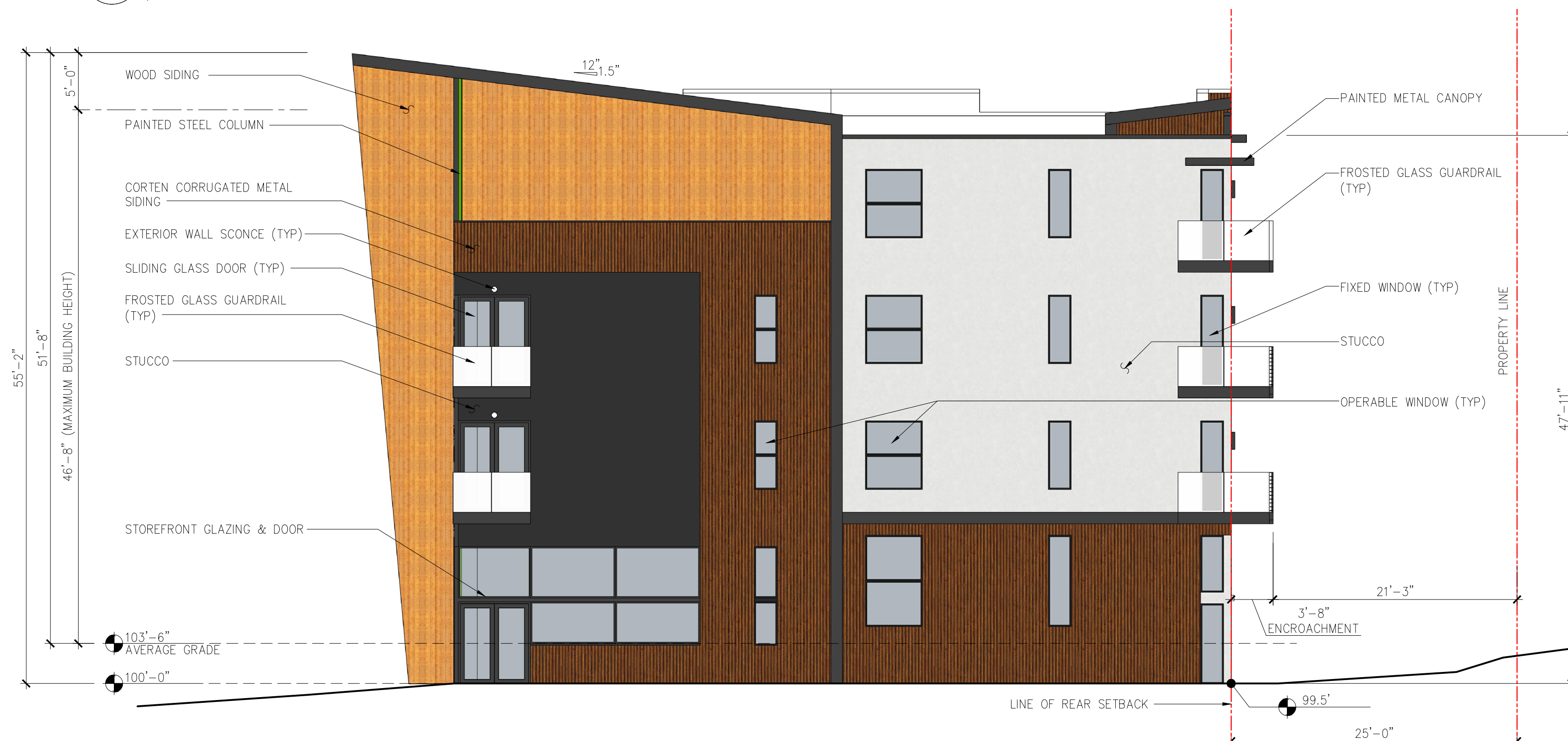
1 NORTH EXTERIOR ELEVATION 1/8"=1'-0"
