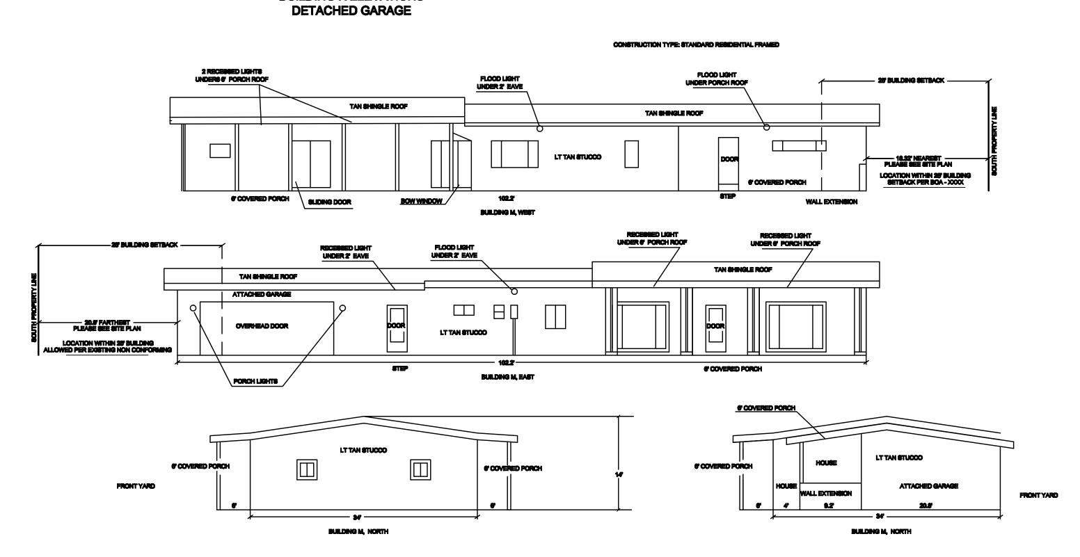
**BUILDING M ELEVATIONS** OFFICE, DRY STORAGE, ATTACHED GARAGE
