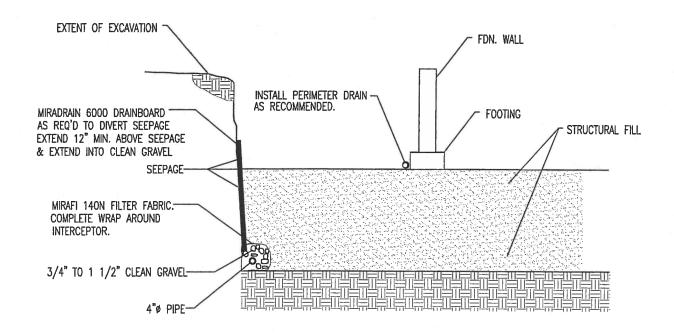
NOTE: EXTEND INTERCEPTOR DRAIN TO DAYLIGHT
