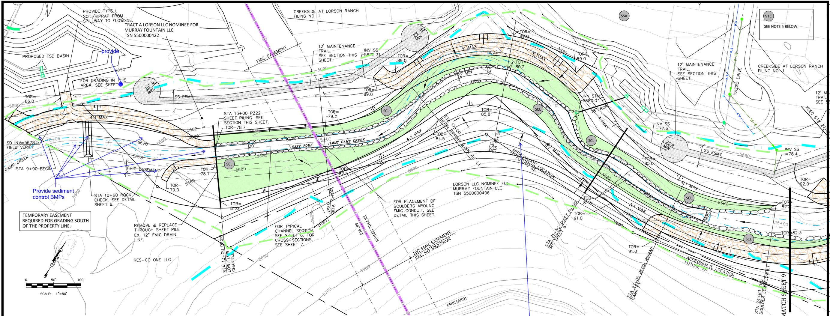
TEMPORARY EASEMENT REQUIRED FOR GRADING SOUTH OF THE PROPERTY LINE.
