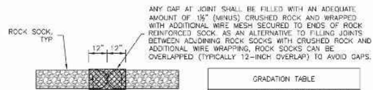
ROCK SOCK JOINTING
