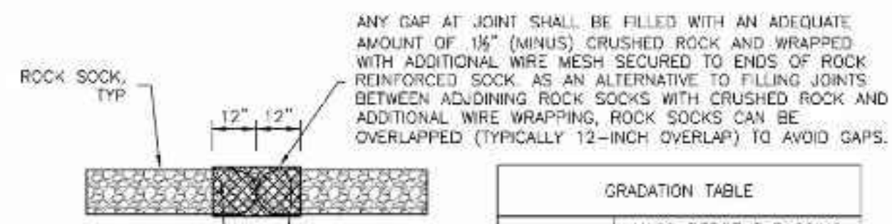
ROCK SOCK JOINTING
