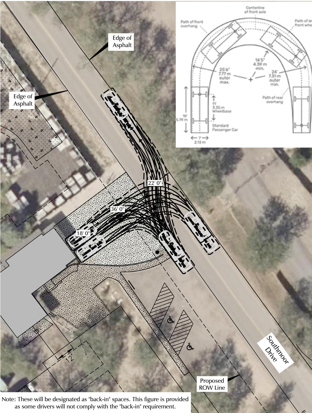
Note: These will be designated as "back-in" spaces. This figure is provided as some drivers will not comply with the "back-in" requirement.
