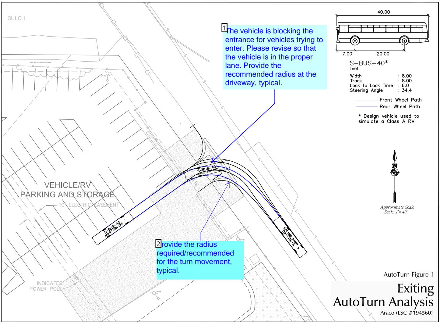
1 The vehicle is blocking the entrance for vehicles trying to enter. Please revise so that the vehicle is in the proper lane. Provide the recommended radius at the driveway, typical.
