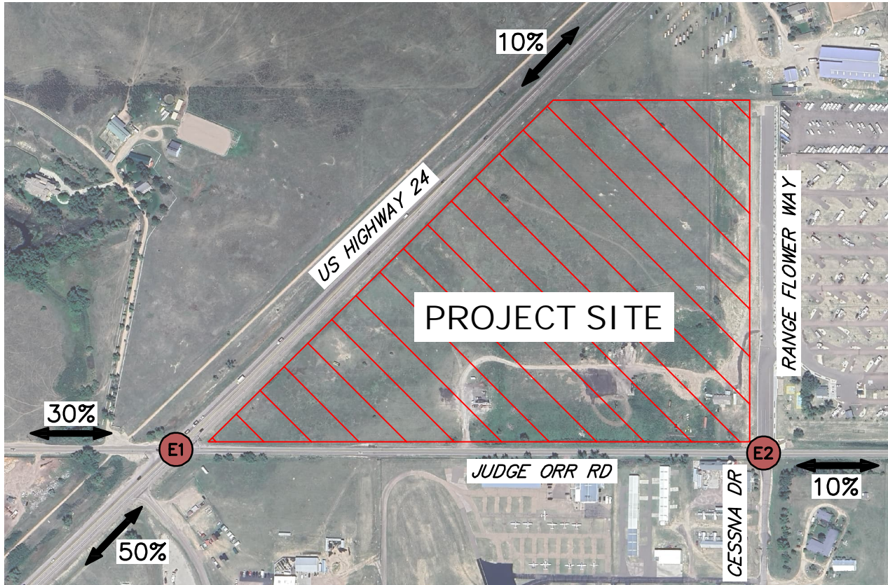
Figure 3 - Site Generated Traffic Volumes and Distribution
