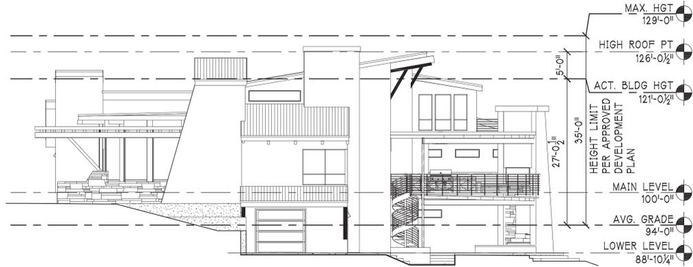
3 NORTH ELEVATION - MAX. BLDG HGT
