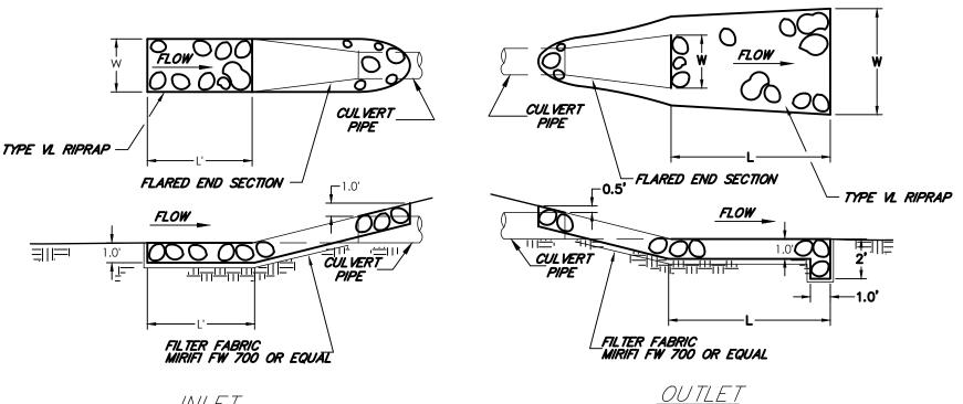
RIPRAP AT CULVERT ENDS Dimensions do not match field measurements. See Stormwater Punchlist, dated 10.25.2023 and revise accordingly. Provide calculations for any outlet
