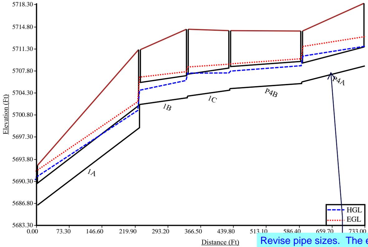
Revise pipe sizes. The entire section is under pressure.
