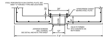
**OUTLET STRUCTURE AT ORIFICE PLATE DETAILS**
